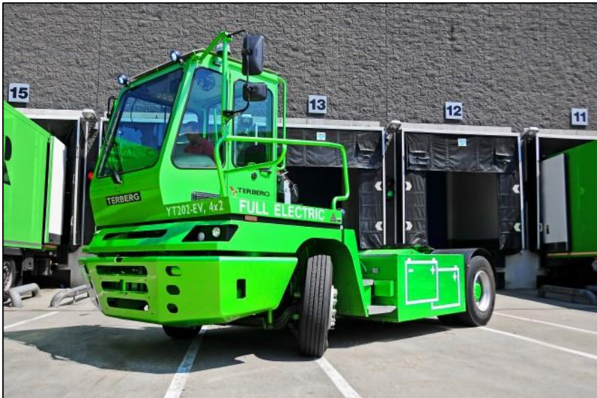
Figure 9-11: Terberg YT202-EV, terminal tractor with electric propulsion(Terberg, 2018).
