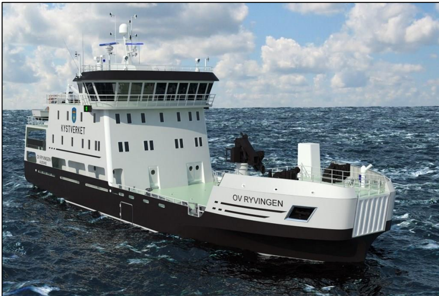
Figure 9-13: The Norwegian Coastal Administration’s “OV Ryvingen”, to be delivered in autumn 2018, has a range of innovative solutions installed on board, including a plug-in hybrid propulsion system, a “thermos” for providing steam and Electric steam boilers (Teknisk Ukeblad, 2018).
