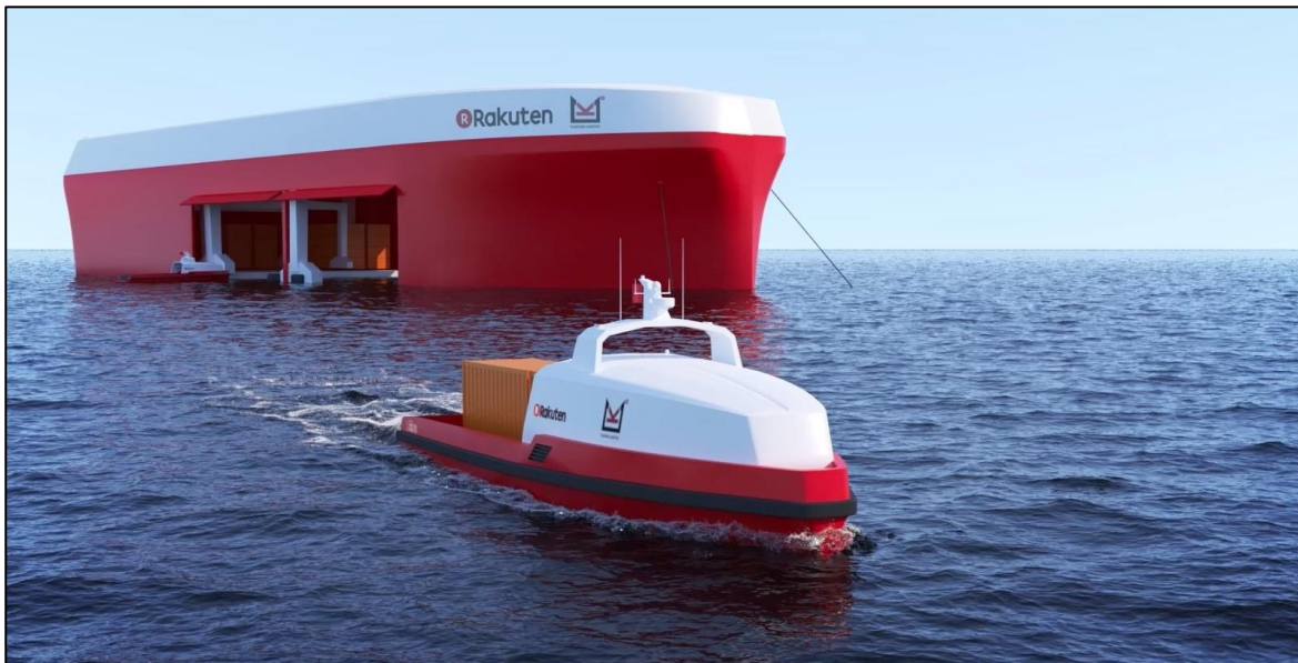
Figure 9-10: The 22-metre-long concept ship K22, designed to carry two 20-foot containers (Teknisk Ukeblad, 2018).
